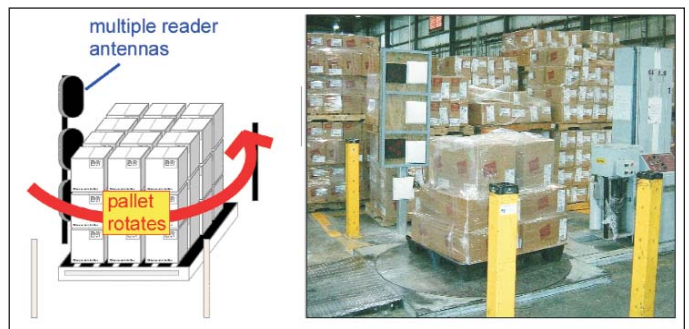
Figure 24 · Schematic depiction of rotating x-ray pallet read (left) and photograph of typical installation (right).
