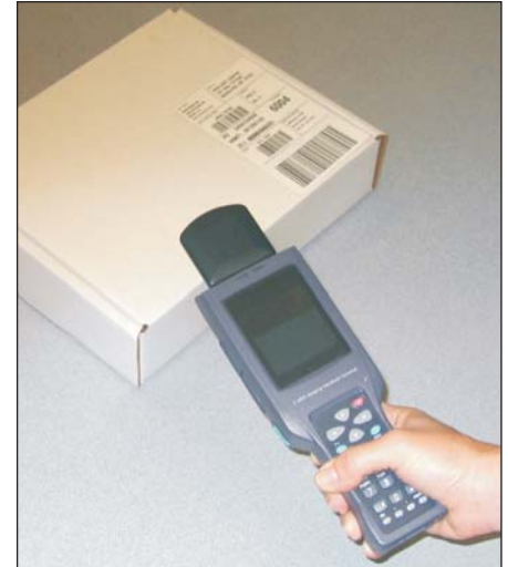
Figure 28 · Handheld RFID reader using removable PC-card RFID module.
