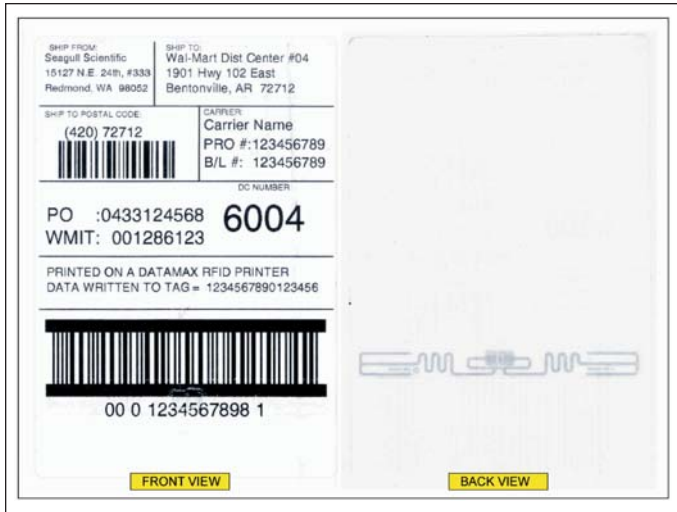
Figure 22 · Front and back views of a human-readable label with embedded RFID tag.
