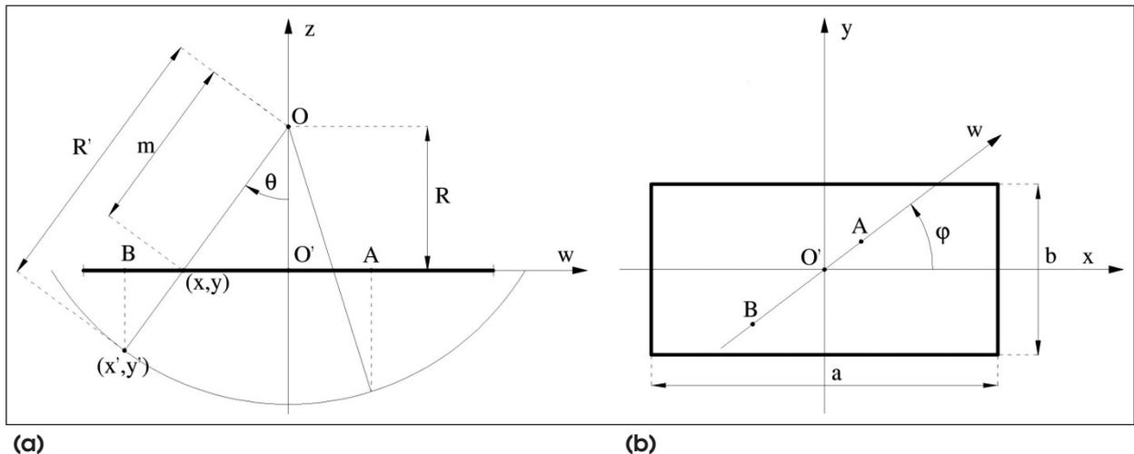
Figure 3 • Cross-sections of a flat, rectangular reflector with feed placed at O.
