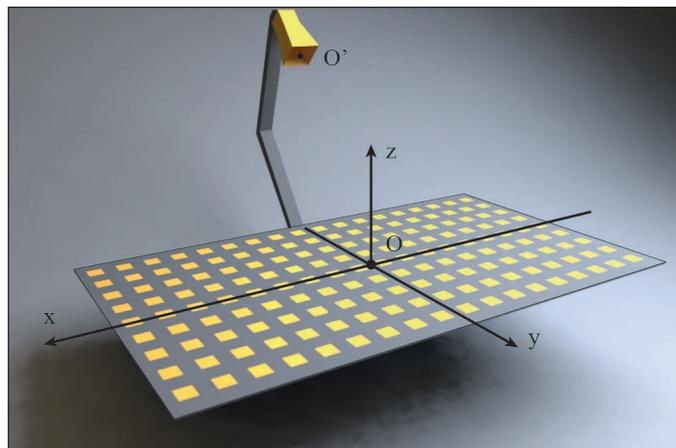
Figure 1 • Reflectarray schematic with reflectarray elements and feed marked in yellow.
