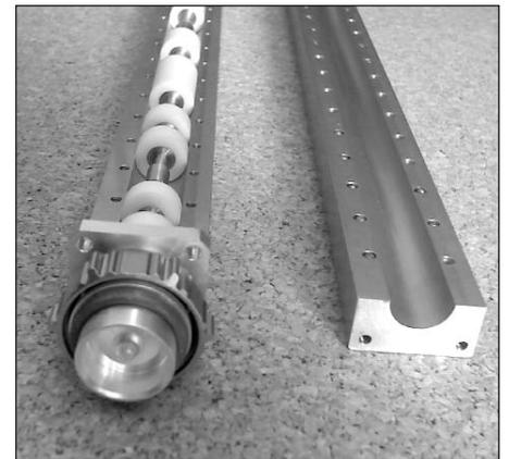
Figure 18 · Construction outline of Filter III.
