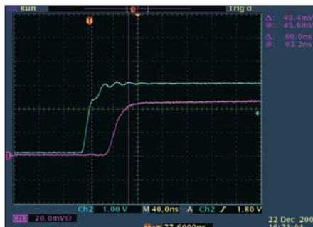
Figure 8 · This is the turn on time of the LNA enable (VREF) using the second method (diode detector). The typical turn on time is ~27 ns.
