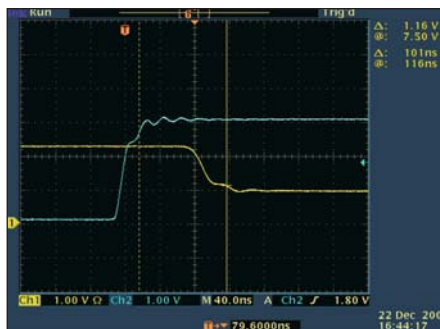
Figure 5 · This is the turn on time of the gain select (bypass mode) using the first method. When this function is exercised it means that the LNA is now in bypass mode and the typical insertion gain is around 3 dB. The typical turn on time is ~100 ns.
