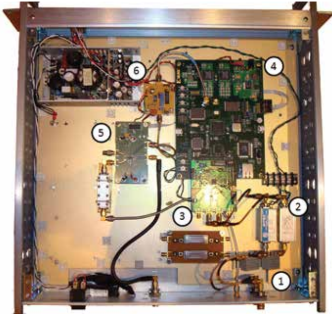
Figure 3 • FPGA – based receiver and sweep- source. (1) 60 MHz, 8 MHz BW filters. (2) 30 dB IF amplifiers. (3) Hittite HMCAD 1520 evaluation board. (4) Xilinx SP601 FPGA evaluation board. (5) Linear Technologies 6946-3 PLL/VCO evaluation board. (6) Reference digitizer.
