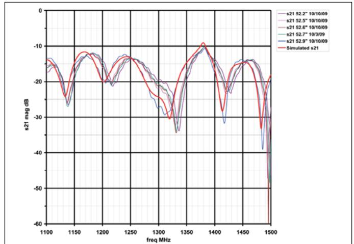
Figure 17 · Measured  $S_{21}$  of the feed with an actual 12 foot dish, compared with the simulation.
