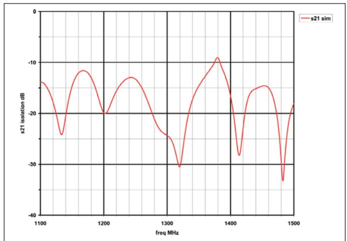
Figure 7 · Simulation of  $S_{21}$  (isolation) of the feed with a 12 ft dish.
