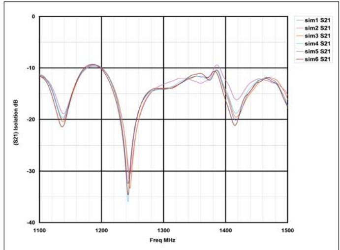
Figure 3 · Comparison of six  $S_{21}$  simulations of the feed with a 10 lambda dish.
