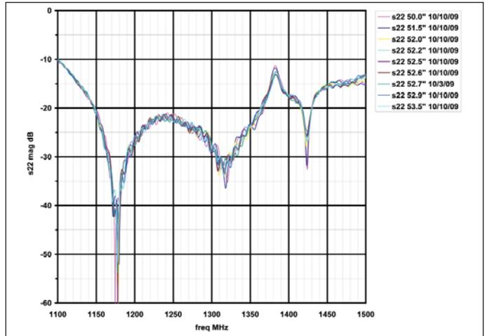
Figure 11 · Measured  $S_{22}$  of the feed with an actual 12 foot dish, placed at various distances from the vertex.
