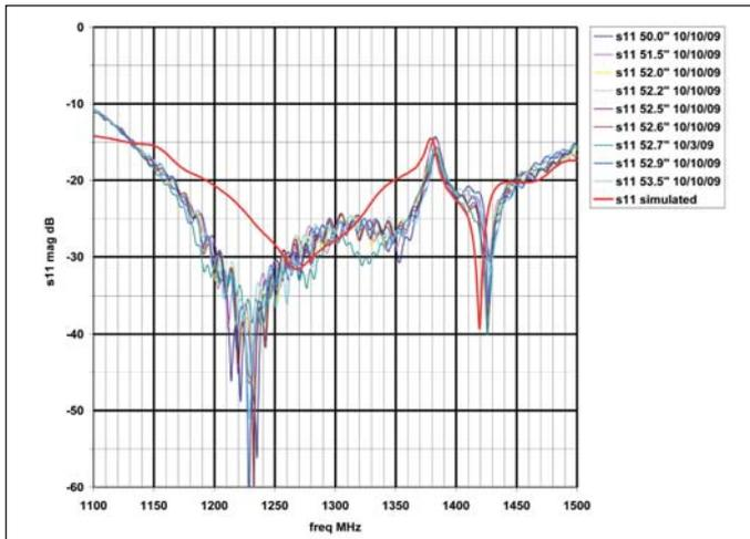
Figure 12 · Measured  $S_{11}$  of the feed with an actual 12 foot dish, placed at various distances from the vertex, compared with the simulation.
