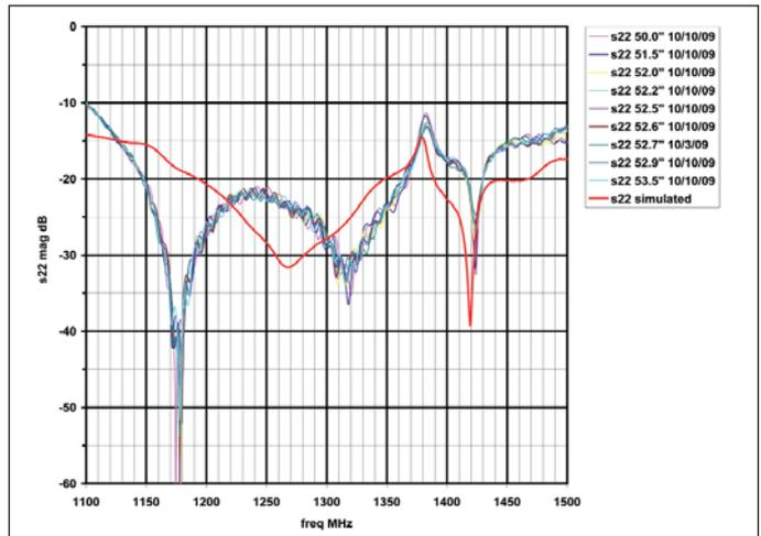
Figure 13 · Measured  $S_{22}$  of the feed with an actual 12 foot dish, placed at various distances from the vertex, compared with the simulation.
