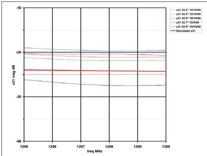
Figure 18 · Measured  $S_{21}$  of the feed with an actual 12 foot dish at various distances from the vertex, compared with the simulation, over a narrow range around the desired operating frequency.
