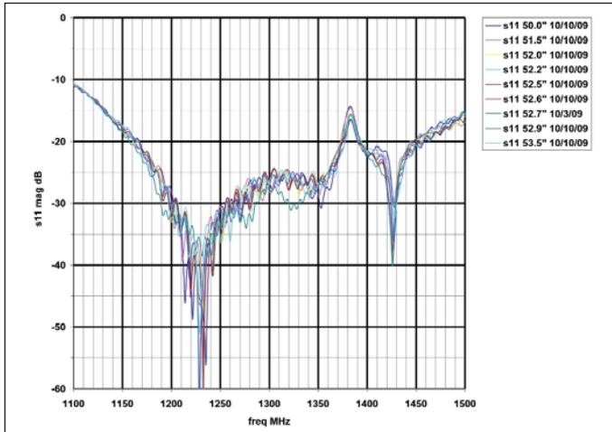
Figure 10 · Measured  $S_{11}$  of the feed with an actual 12 foot dish, placed at various distances from the vertex.
