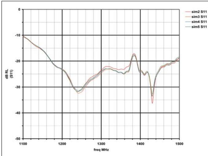
Figure 2 · Comparison of four  $S_{11}$  simulations of the feed with a 10 lambda dish.
