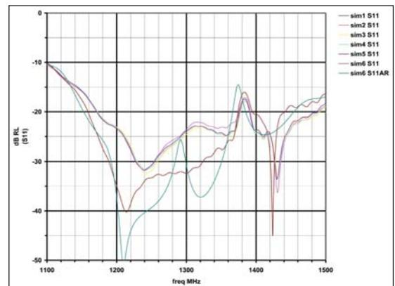
Figure 1 · Comparison of six  $S_{11}$  simulations of the feed with a 10 lambda dish.
