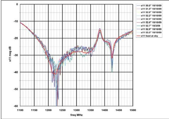
Figure 14 · Measured  $S_{11}$  of the feed with an actual 12 foot dish, placed at various distances from the vertex, compared with measurement of the feed pointed at open sky.
