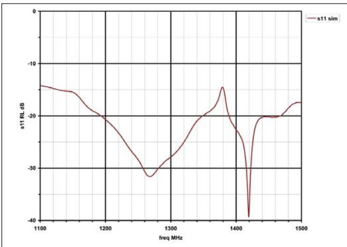
Figure 6 · Simulation of  $S_{11}$  (RL) of the feed with a 12 ft dish.
