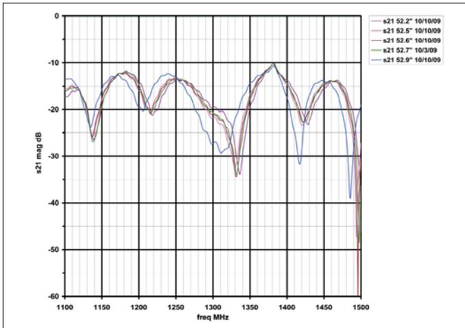
Figure 16 · Measured  $S_{21}$  of the feed with an actual 12 foot dish, place at various distances from the vertex.
