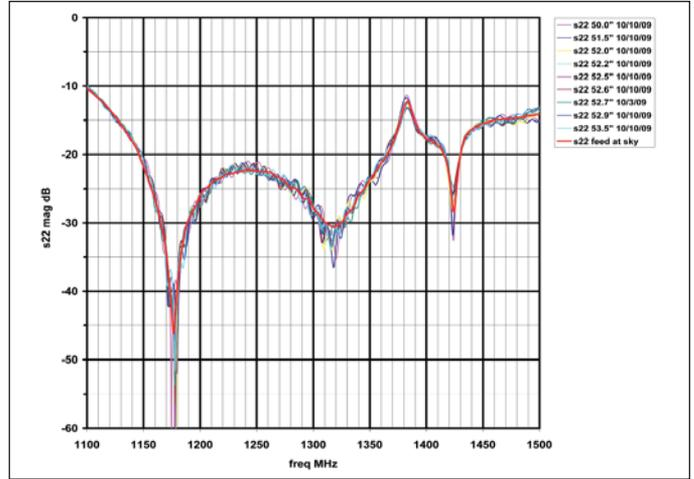
Figure 15 · Measured  $S_{22}$  of the feed with an actual 12 foot dish, placed at various distances from the vertex, compared with measurement of the feed pointed at open sky.
