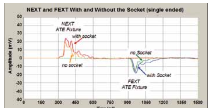
Figure 13 • ATE DUT Board NEXT and FEXT crosstalk between adjacent BGA connections with and without the BGA socket in the signal path.
