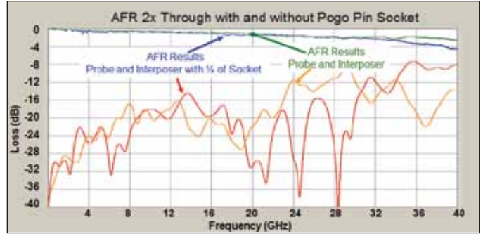
Figure 10 • Alternative AFR calibration using a 2x through path to measure the Probe Interposer.
