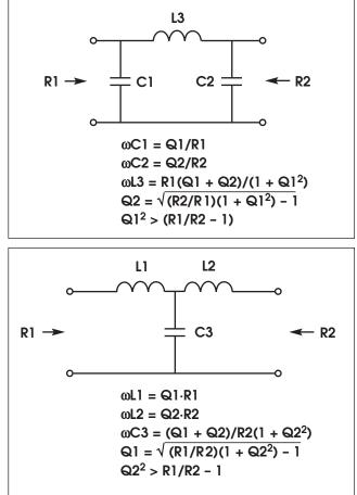
Additional topologies are possible, with inductors or capacitors in each position. These two are shown as examples. Readers are referred to texts on matching networks for additional information.
