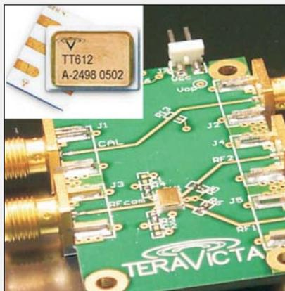
**Dow-Key Microwave** offers MEMS switches from **Teravicta Technologies**. The switches provide low-loss performance of 0.1 dB at 1 GHz, 0.3 dB at 6 GHz, with a frequency response down to 300 kHz. The small size and superior performance of MEMS switches will find applications in communications, test, military and aerospace systems.
