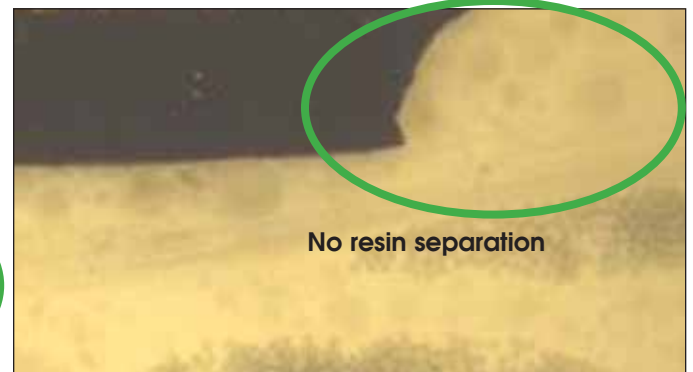
Figure 3 • These high-magnification photos compare the same circuit construction, with resin separation on the left using a low-flow prepreg material. This resin separation does not occur on the right using an optimized prepreg material.
