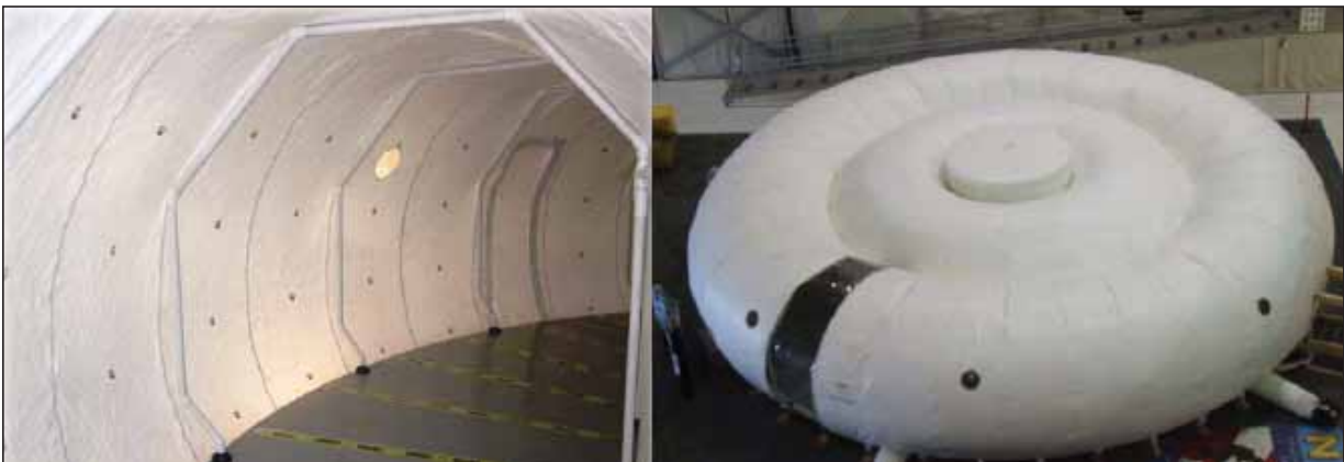
Figure 3 • NASA's Inflatable Lunar Habitat Module at UMaine.
