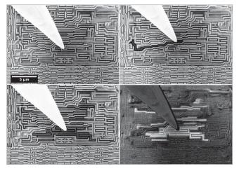
**Fig. 4.** Selective biasing of adjacent interconnects. Top left: Before tip contact. Top right and bottom left: contacting two adjacent lines. Bottom right: Difference image between the two images on the left.
