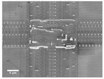
Fig. 1. Passive voltage contrast on an integrated circuit.
