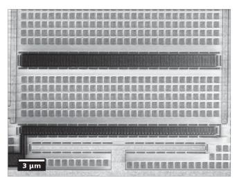
**Fig. 5.** Closed circuit biasing of contact chain structures using two tips (Tips not show in the image). The voltage drop along the chain structures becomes visible as a gradual decrease of voltage contrast.
